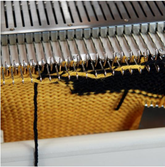
You should be able to see the floats below the needles. They are not long enough to be a problem. Before placing the yarn for the next row, I would catch the black behind the shaft of the last needle at the right of the yellow group. Because the yellow will travel to the right, alternating needle groups with the black, twisting them at this first junction won't prevent a gap.
